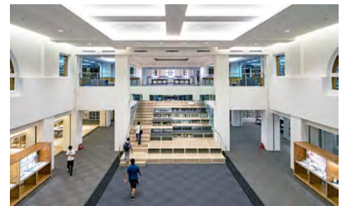
The new main staircase welcomes all readers with an uplifting visual impact; the see-through structure admits sunlight from the rear windows for enhanced lighting. The exhibition area is located above the staircase and the reading area is located below.
