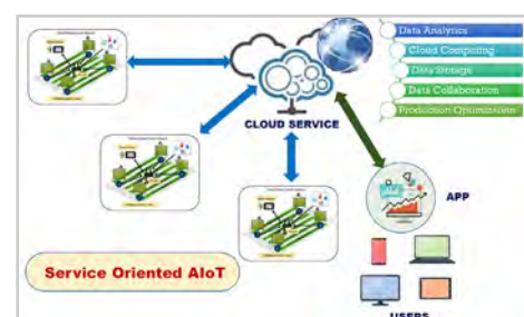
The architecture of the Smart Pest Monitoring System and its digital services.
