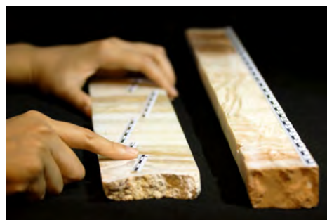
Limestone core samples collected from Bàsura Cave, northern Italy. The black-and-white alternating bands represent a scale measured in centimeters. Researchers follow the scale in extracting small subsamples ranging from 0.1 to 100 milligrams for carbon and oxygen isotope analysis, trace element determination, and uranium-thorium dating.
