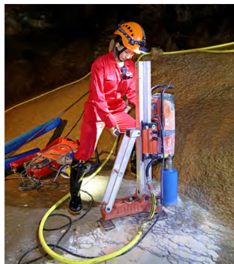
Graduate student Wen-Hui Sung of the Department of Geosciences, National Taiwan University, operating a drilling machine to extract limestone core samples in Bàsura Cave, northern Italy.
