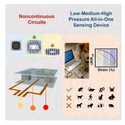
The use of multiple elastic pressure-sensing units containing noncontinuous circuits to innovate a pressure-sensing device with ultra-wide rang
