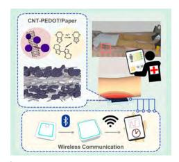
The CNT-PEDOT composite gradient distributed paperbased pressure sensing device with the combined function of remote monitoring for long-term PI prevention.
