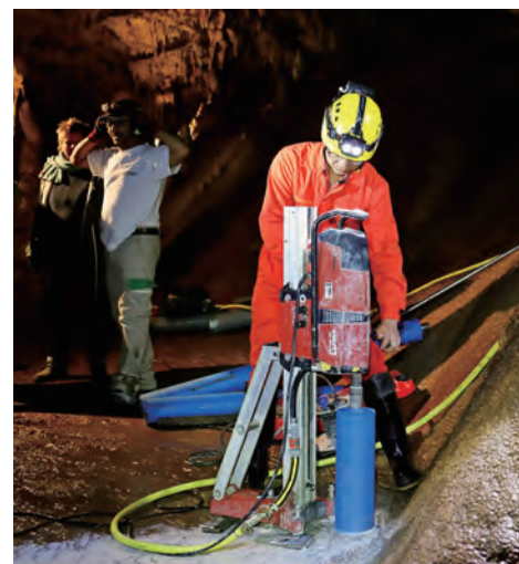
Prof. Chuan-Chou Shen of the Department of Geosciences, operating a core drill rig to extract limestone core samples in Bàsura Cave, in northwestern Italy.
