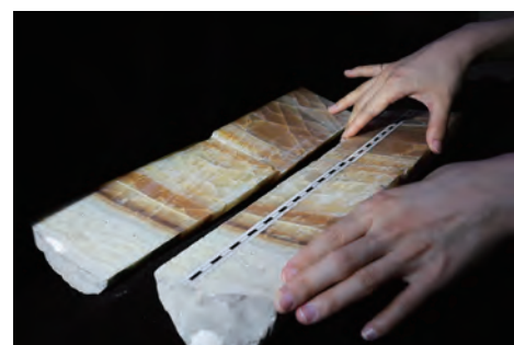
Limestone core samples collected at Bàsura Cave. The black-and-white alternating bands represent a scale measured in centimeters. Researchers follow the scale in extracting small subsamples ranging from 0.1 to 100 milligrams for carbon and oxygen isotope analysis, trace element determination, and uranium-thorium dating.
