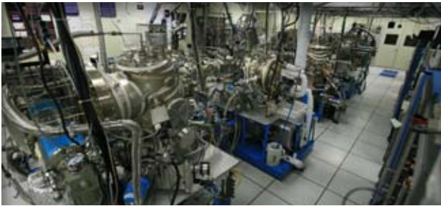
Ⓐ The ultra-high vacuum multi-chamber molecular beam epitaxy (MBE) system at the nano-epitaxy lab
