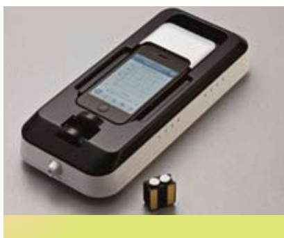
This tricorder allows diabetes patients to detect the density of HbA1c in their blood.
